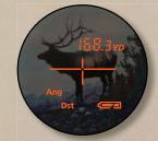
In darker conditions, the rangefinder will automatically turn on the orange LED illumination to the liquid crystal characters for optimum visibility—even adjusting its brightness as needed for appropriate contrast against the background.
