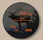
In darker conditions, the rangefinder will automatically turn on the orange LED illumination to the liquid crystal characters for optimum visibility—even adjusting its brightness as needed for appropriate contrast against the background.
